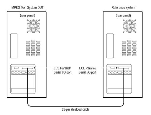
Figure 4–17: Setup for checking ECL parallel port data transfer
