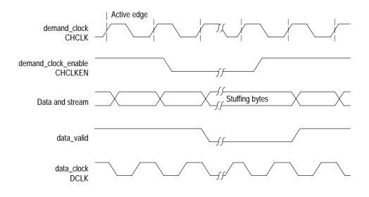
Figure 1–6: ECL Timing diagram with control port
