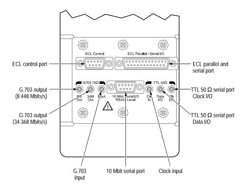
Figure 2–5: Data Store input and output ports
