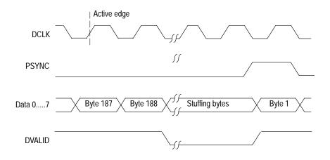
Figure 1–3: Parallel data timing, 188-byte packets
