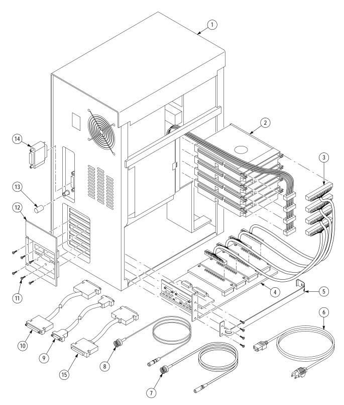
Figure 8–1: MTS100 MPEG Test System
