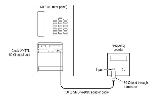
Figure 5–3: Setup for adjusting the clock frequency
