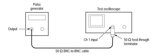
Figure 4–15: Setup for measuring the pulse generator output
