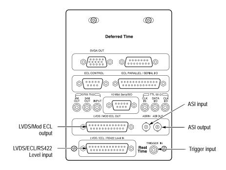
Figure 2-6: Real-Time Analyzer input and output ports (computer rear)
