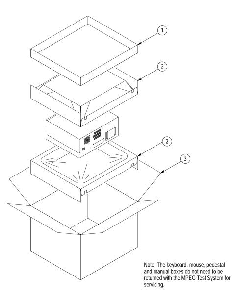
Figure 6–10: Packing illustration
