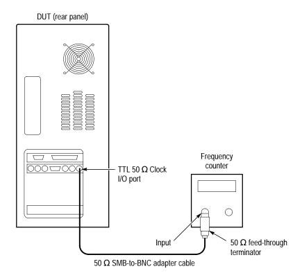
Figure 4–1: Setup for measuring internal clock output accuracy
