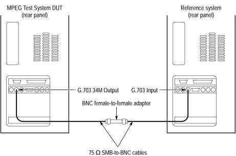
Figure 4-8: Setup for testing G.703 34.368 Mbits/s master generation
