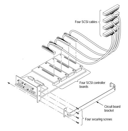
Figure 6–2: Removing the Data Store circuit board
