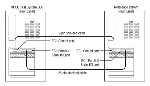
Figure 4–20: Setup for checking ECL parallel port master acquisition and slave generation
