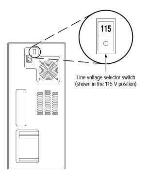
Figure 2–2: Server voltage selection switch
