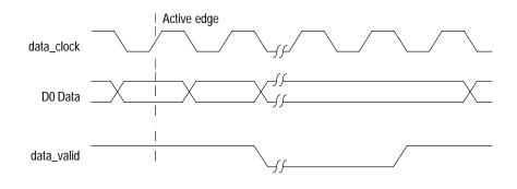
Figure 1–5: Timing diagram for the ECL serial port
