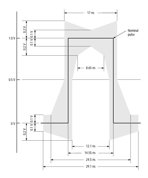
Figure 1–2: Pulse specification for a G.703 34.368 MHz pulse
