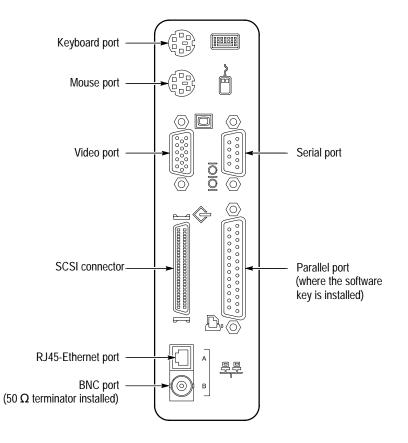
Figure 2–3: The rear panel of the server
