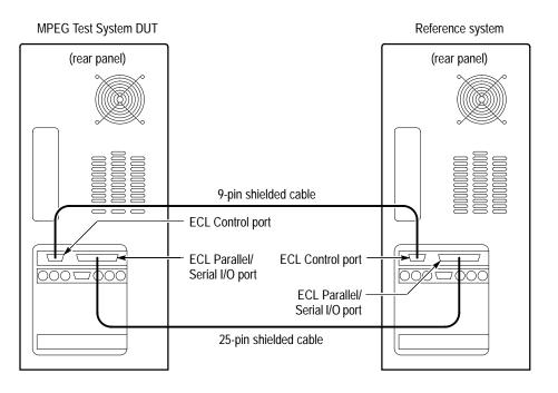
Figure 4–24: Setup for checking ECL serial port slave generation
