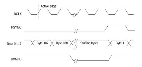
Figure 1–9: Parallel data timing, 188-byte packets
