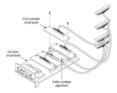
Figure 5–1: Location of the 8.448 MHz oscillator adjustment
