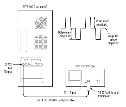
Figure 4–2: Setup for measuring 8 Mbits/s signal parameters
