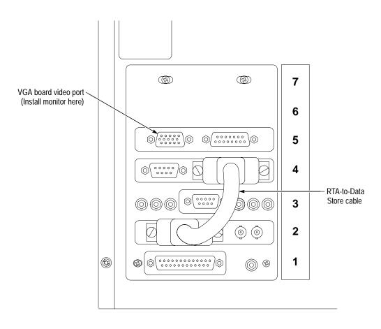
Figure 2–7: RTA output to Data Store input connection
