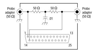
Figure 4–26: Breakout box for LVDS port tests
