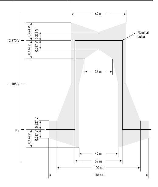
Figure 1–1: Pulse specification for a G.703 8.448 MHz pulse
