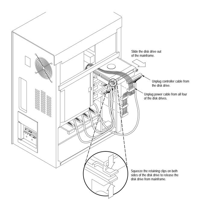
Figure 6–3: Removing Data Store hard disk drives
