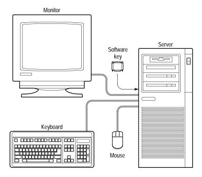
Figure 2–1: The MTS100 MPEG Test System
