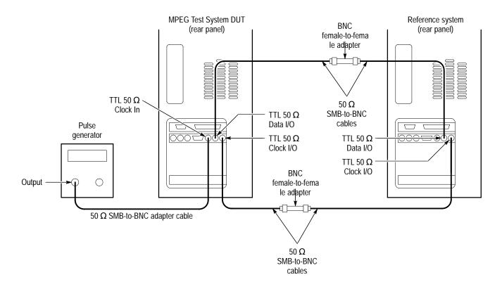
Figure 4–12: Setup for checking 50 ohm external clock generation
