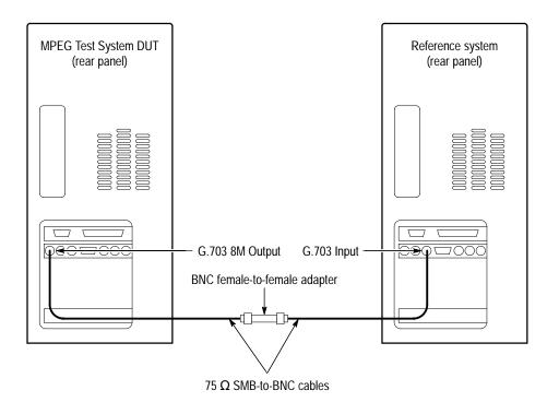
Figure 4–5: Setup for testing G.703 8.448 Mbits/s master generation
