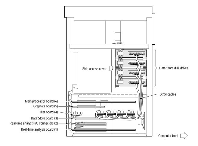
**5.** Lift up and remove the panel to gain access to the server side access bays and EISA card cage. See Figure 6–1.
