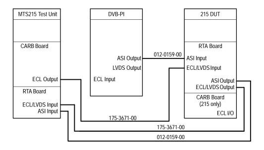
Figure 4–28: Hardware connections for verifying Modified ECL input
