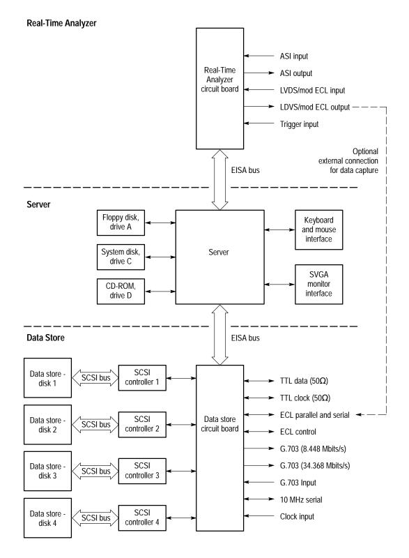
Figure 3–1: Test System block diagram
